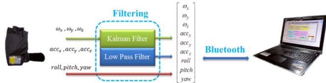
Fig. 5. Filtering of IMU data.
