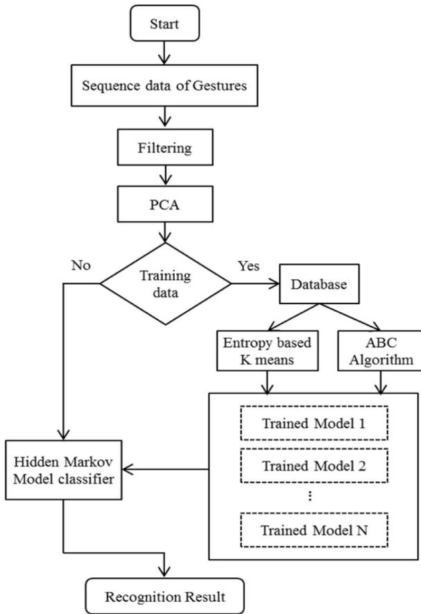
Fig. 2. System diagram of TSL Recognition.
