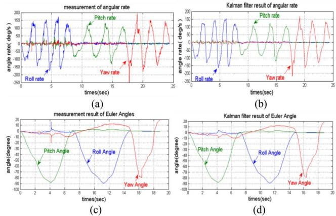
Fig. 4. (a) Raw Gyro data of the sensor. (b) Kalman filter result of the Gyro data acquired by rotating the sensor between  $0^\circ$  and  $-90^\circ$  in three axes by hand. (c) Raw Euler angle data. (d) Kalman filter result of Euler angle.
