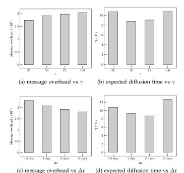
Fig. 5: Performance of *Set-cover* with varying  $\gamma$  and  $\Delta t$  in terms of message overhead and expected diffusion time, where k=50,  $\Delta t=2$  days for (a) and (b), and k=50,  $\gamma=50$  for (c) and (d).
