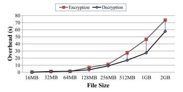
Fig. 7. Comparisons of overhead for encryption and decryption.
