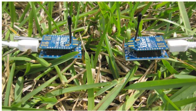
Fig. 2. Nodes orientation for vertical polarization on the ground in short grass terrain.
