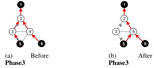
Fig. 3. An example of removing successive links in a tree. The arcs with X sign denote the removed tree links.
