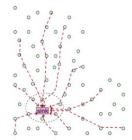
Fig. 1. Tree topology static WSN with a multi-hop communication network.
