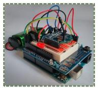
Fig. 4. ZED developed for the ZigBee WDSN proof of concept.
