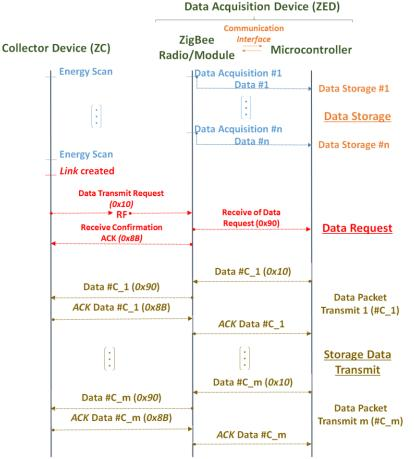
Fig. 3. Implementation guide: communication diagram of peer-to-peer WDSN
