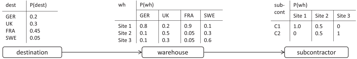
Figure 4. Bayesian Network consisting of Topology and Conditional Probability Tables
