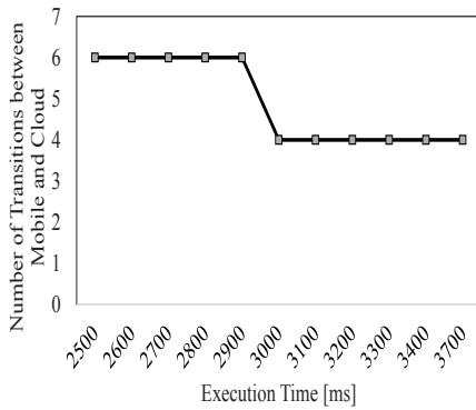
Fig. 9: Number of transitions between the mobile and cloud for offloading in correspondence with execution time ( T ) while R_u=0.8\text{Mbps} and R_d=1.76\text{Mbps} .
