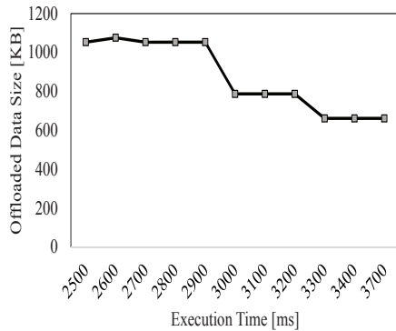
Fig. 10: Allocated data size for cloud offloading in correspondence with execution time ( T ) while R_u=0.8\text{Mbps} and R_d=1.76\text{Mbps} .
